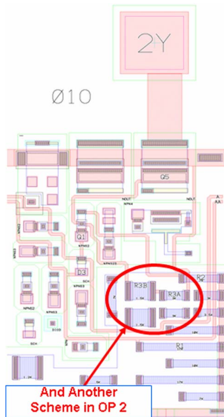
Figure 7 Physical Layout of Output Structure 2
