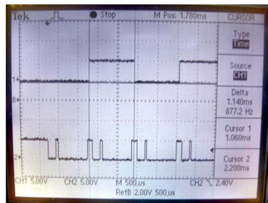
Figure 7. Data I/O A0 Program - showing LSB address pin and Pgm pulse
